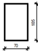
$$\begin{aligned} A &= 0.735 \text{ m}^2 \\ I_y &= 0.068 \text{ m}^4 \\ I_z &= 0.030 \text{ m}^4 \\ E &= 35000 \text{ MPa} \end{aligned}$$
