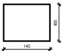
$$\begin{aligned} A &= 1.47 \text{ m}^2 \\ I_y &= 0.135 \text{ m}^4 \\ I_z &= 0.240 \text{ m}^4 \\ E &= 35000 \text{ MPa} \end{aligned}$$
