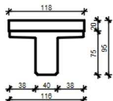
$$\begin{aligned} A &= 0.618 \text{ m}^2 \\ I_y &= 0.045 \text{ m}^4 \\ I_z &= 0.045 \text{ m}^4 \\ E &= 35000 \text{ MPa} \end{aligned}$$
