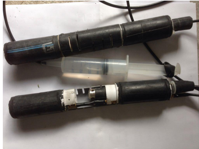
FIGURE A.21: Borehole packers.
