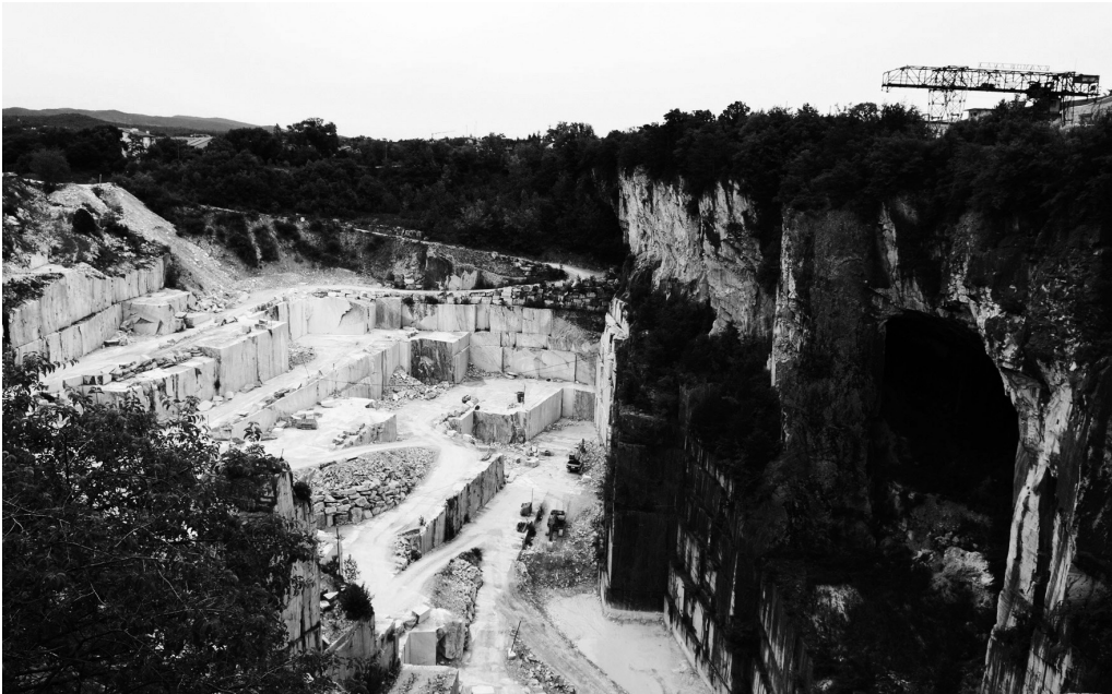
Fig. 4. Aurisina (Trieste, Italy). The Cava Romana quarry. On the right, the tunnel exploited in ancient times. On the left, the active quarry
