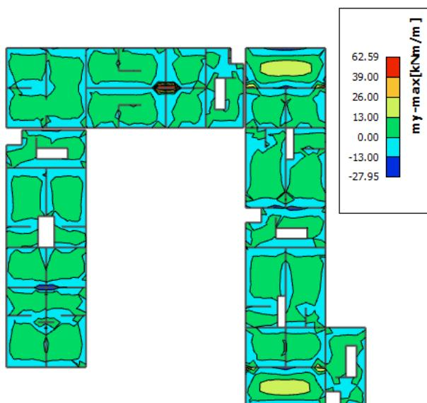
**$M_y$  (ostali dijelovi ploče)**
