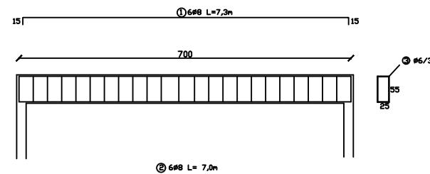
POPREČNI PRESJEK - PRIKAZ ARMATURE
