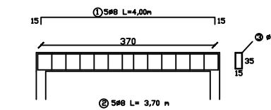
POPREČNI PRESJEK - PRIKAZ ARMATURE
