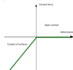
Stress-strain diagram of contact between the concrete block and the base plate
