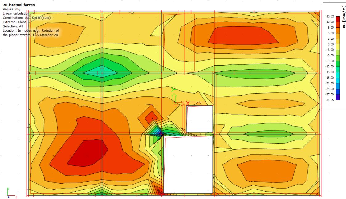
Slika 58 2D dijagram momenata savijanja  $M_y$
