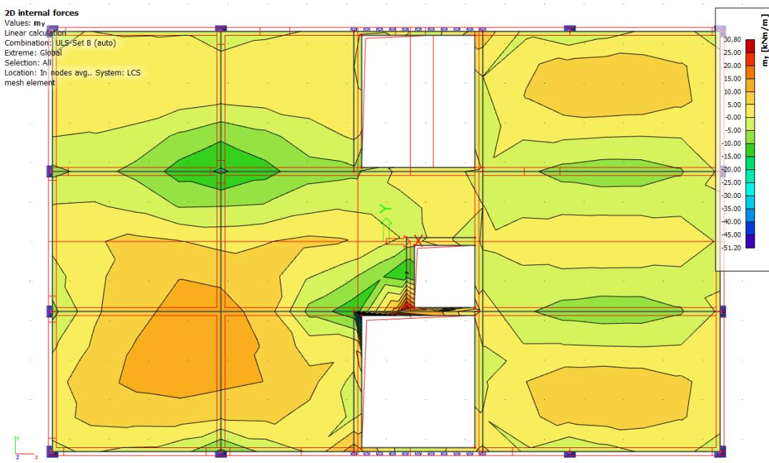
Slika 66 2D dijagram momenata savijanja  $M_y$
