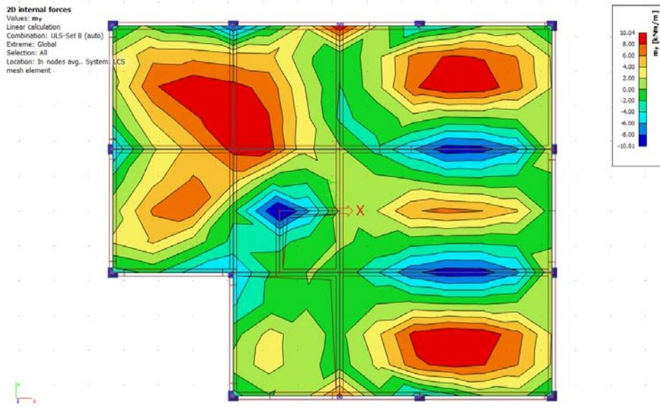
Slika 48 2D dijagram momenata savijanja  $M_y$
