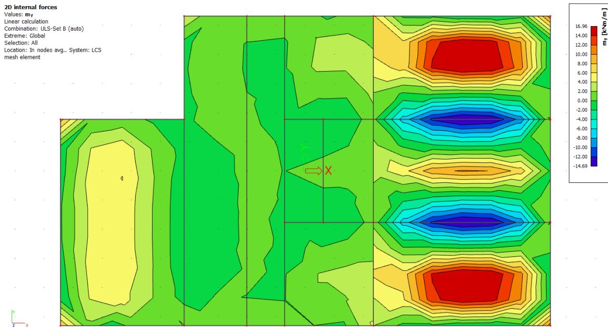
Slika 82 2D dijagram momenata savijanja  $M_y$
