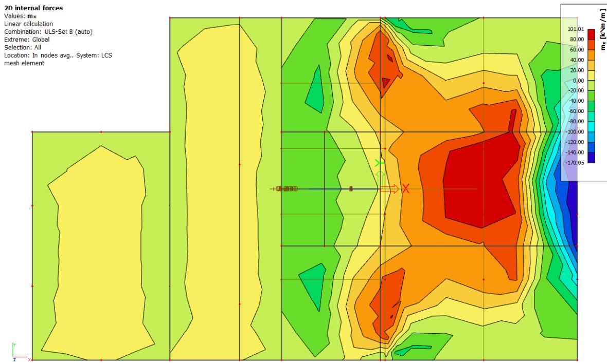
Slika 84 2D dijagram momenata savijanja  $M_x$
