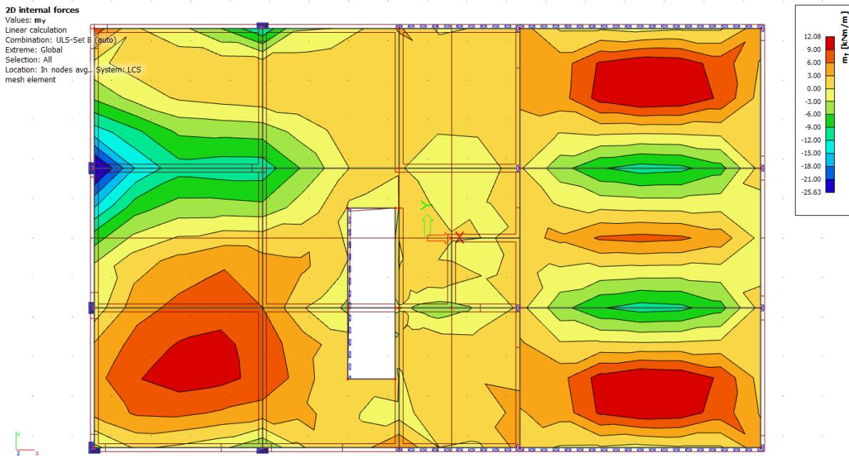
Slika 74 2D dijagram momenata savijanja  $M_y$
