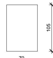
$$\begin{aligned} A &= 0,735 \text{ m}^2 \\ I_y &= 0,068 \text{ m}^4 \\ I_z &= 0,030 \text{ m}^4 \\ E &= 35000 \text{ MPa} \end{aligned}$$
