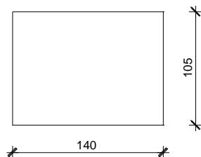
$$\begin{aligned} A &= 1,47 \text{ m}^2 \\ I_y &= 0,135 \text{ m}^4 \\ I_z &= 0,240 \text{ m}^4 \\ E &= 35000 \text{ MPa} \end{aligned}$$
