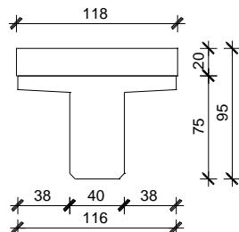
$$\begin{aligned} A &= 0,618 \text{ m}^2 \\ I_y &= 0,045 \text{ m}^4 \\ I_z &= 0,045 \text{ m}^4 \\ E &= 35000 \text{ MPa} \end{aligned}$$
