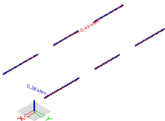
*Slika 7.2.3.3.Moment M<sub>x</sub>***1D internal forces**
