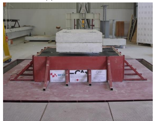
Fig. 3 Adopted model of the rigid building (Banović et al. 2019)
