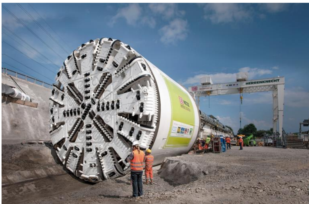
Slika 2.1: Herrenknecht Multi-Mode Tunnel Boring Machine [2]
