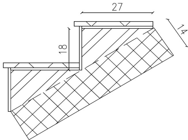
$$\operatorname{tg} \alpha = v_{st} / \dot{v}_{st} = 18/27 = 0,667 ; \alpha=33,69^{\circ}$$
