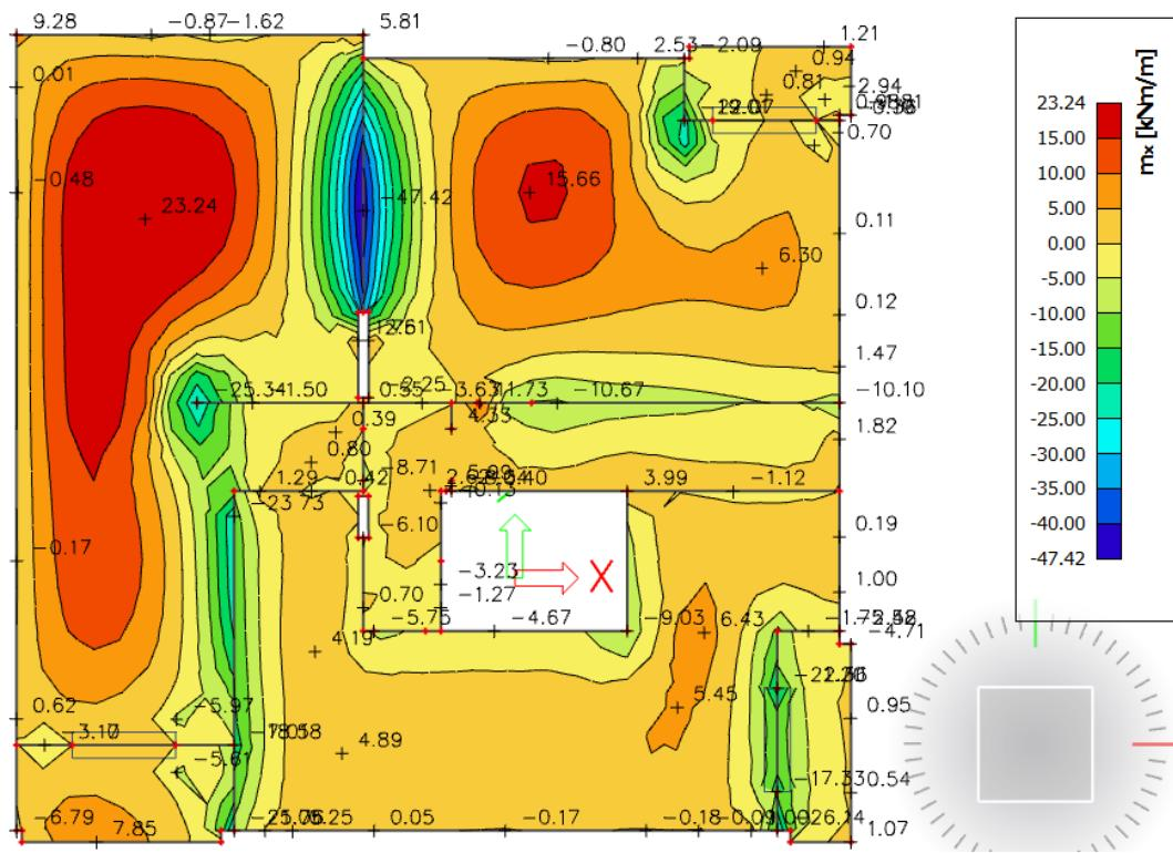
Slika 6.30. Prikaz momenata savijanja u polju  $M_x$  – GSN2
