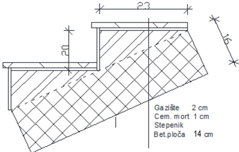
$$\begin{aligned} \operatorname{tg} \alpha &= v_s / s_s = 20 / 23 = 0,8696 ; \alpha = 41.01^\circ \\ h' &= h / \cos \alpha = 14 / \cos 41.01^\circ = 21.20 \text{ cm} \end{aligned}$$
