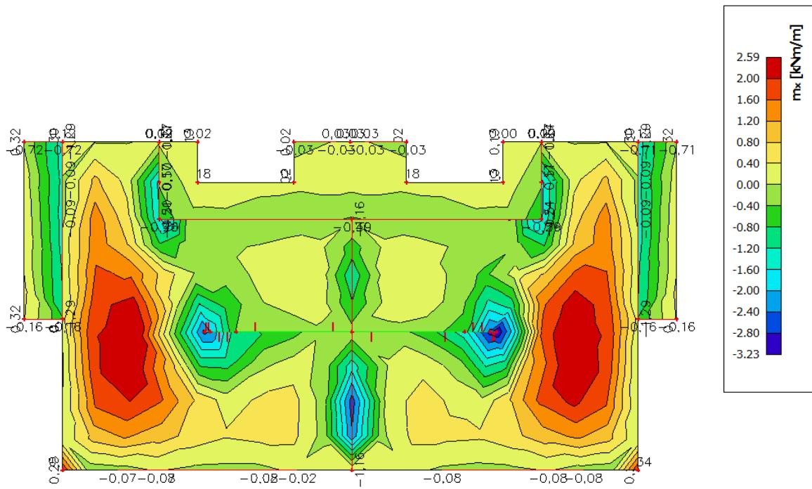
Slika 6.7 Potrebna površina armature  $A_s(\text{cm}^2/\text{m})$  u  $x$  smjeru
