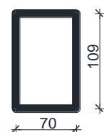
$$\begin{aligned}A &= 0.76 \text{ m}^2 \\I_y &= 10.0 \text{ m}^4 \\I_z &= 0.1302 \text{ m}^4\end{aligned}$$
