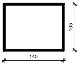
$$\begin{aligned} A &= 1.470 \text{ m}^2 \\ I_y &= 0.240 \text{ m}^4 \\ I_z &= 0.135 \text{ m}^4 \\ E &= 34000 \text{ MPa} \end{aligned}$$
