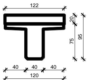
$$\begin{aligned} A &= 0.630 \text{ m}^2 \\ I_y &= 0.023 \text{ m}^4 \\ I_z &= 0.046 \text{ m}^4 \\ E &= 34000 \text{ MPa} \end{aligned}$$
