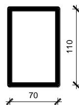
$$\begin{aligned} A &= 0.770 \text{ m}^2 \\ I_y &= 0.031 \text{ m}^4 \\ I_z &= 0.078 \text{ m}^4 \\ E &= 34000 \text{ MPa} \end{aligned}$$
