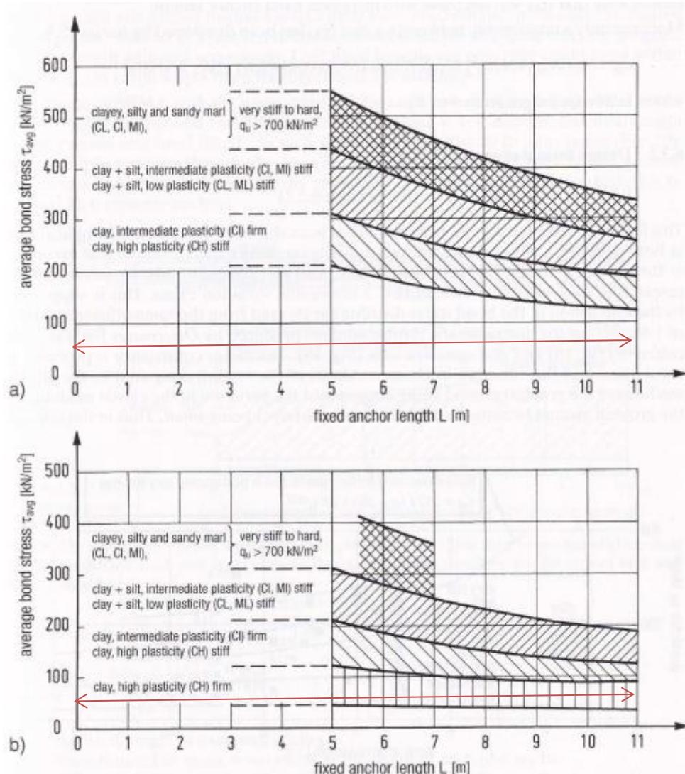
**Fig. 18.** Average bond stress at ultimate limit state of anchors in cohesive soils
