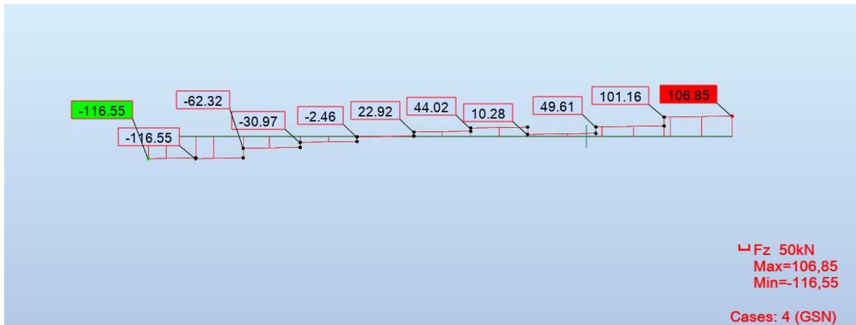
Slika 6.64.  $V_z$  (kN)**SAVOJNI MOMENTI ZA GSU**
