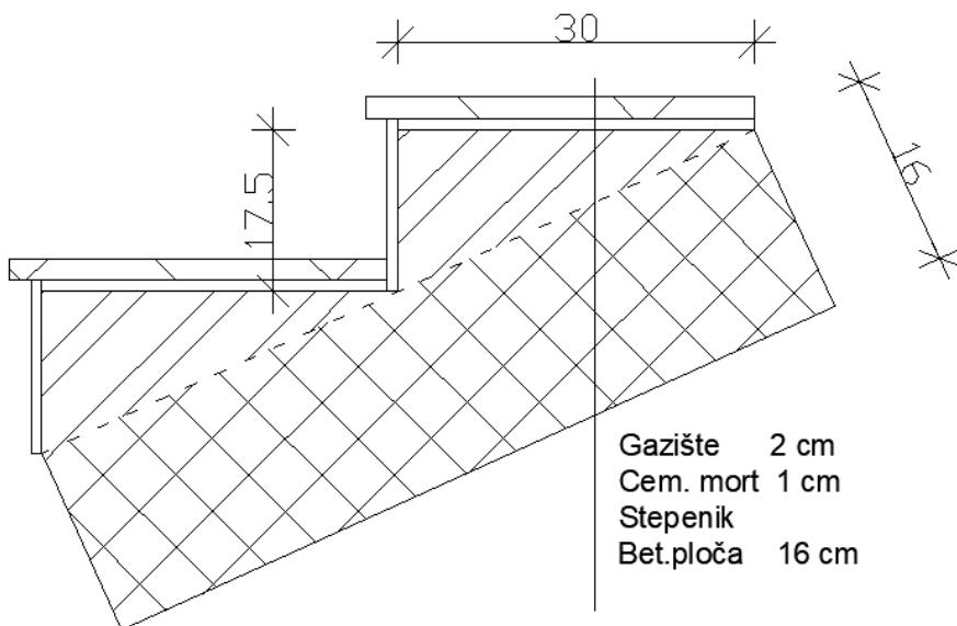
$$\operatorname{tg}\alpha = v_{st} / s_{st} = 17.5 / 30 = 0.6 \quad ; \quad \alpha = 30.26^\circ$$
