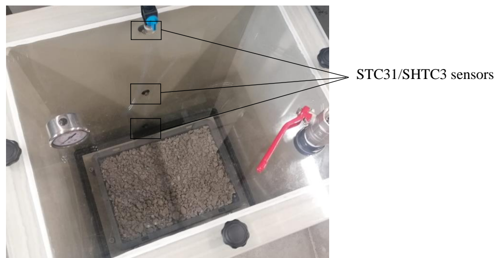
Fig. 32. Sensors inside chamber
