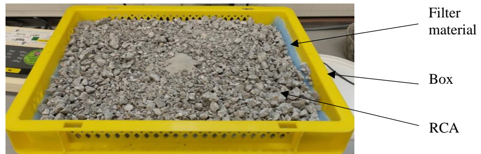
Fig. 27. RCA prepared for CO 2 curing.
