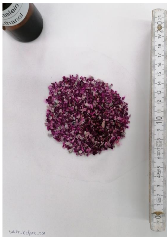
Fig. 10. Phenolphthalein test results before CO 2 curing for experiment WL17.
