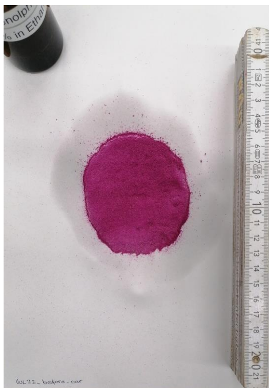
Fig. 25. Phenolphthalein test results before CO 2 curing for experiment WL22.
