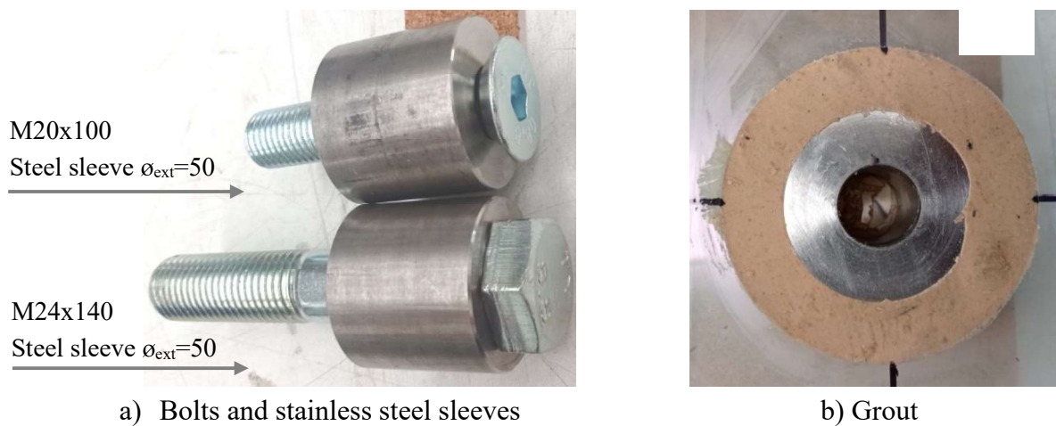
Figure 3.6 – Elements fit in the borehole
