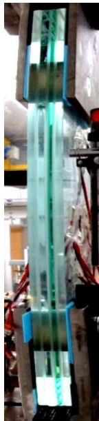
a) Collapse of the 1 st ply (top)
