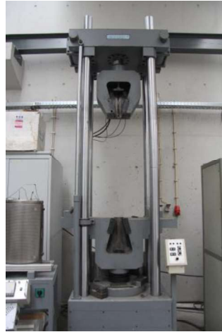
Figure 3.3 – Universal Testing Machine SERVOSIS 80ton [7]
