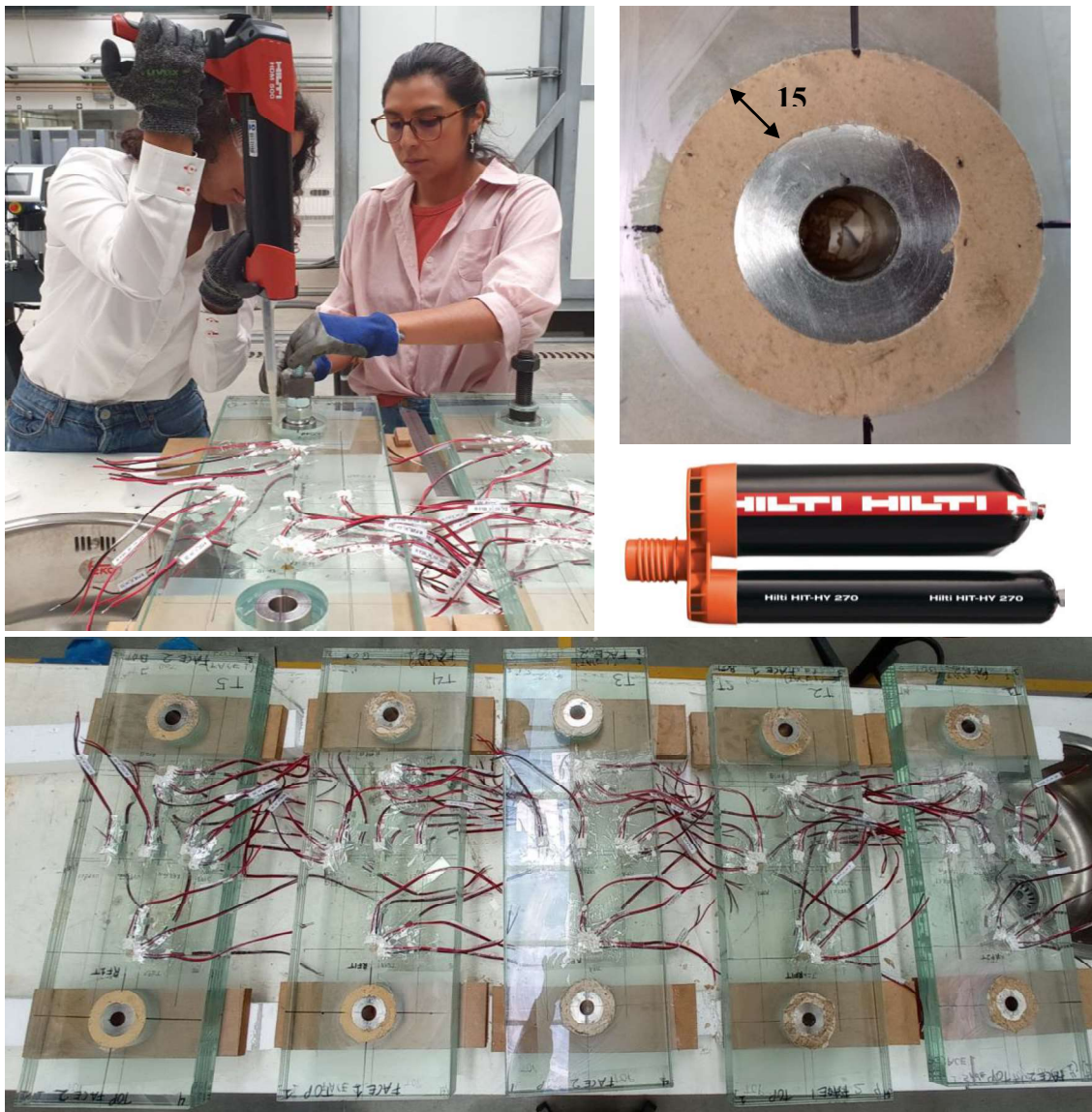
Figure 3.12 – Details regarding the grout application [7]
