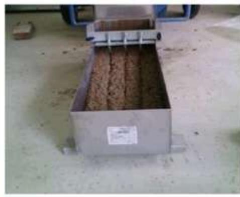
**Fig. 6** L-box: SCLC 4 - sticky mixture
