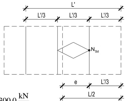
$$\sigma_{ekv} = \frac{2 \cdot (N_{sd} + G)}{L' \cdot B} = \frac{2 \cdot (96,4 + 100,0)}{0,96 \cdot 2,0} = 204,58 \frac{\text{kN}}{\text{m}^2} < \sigma_{tla,lim} = 300,0 \frac{\text{kN}}{\text{m}^2}$$
