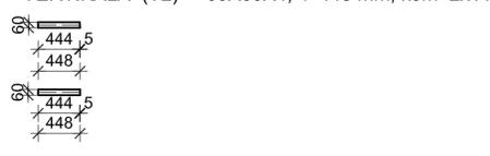
VERTIKALA (V4) 60X60X4, l=898 mm, kom=2x11
