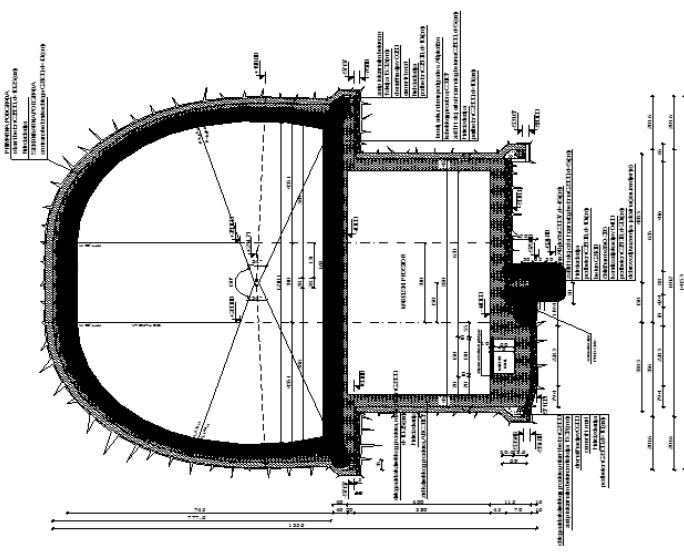
**NORMALNI POPREČNI PRESJECI KABELSKOG TUNELA
