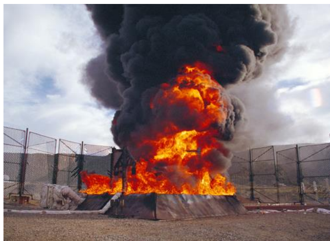
Figure 10: Example of a pool fire [51]
