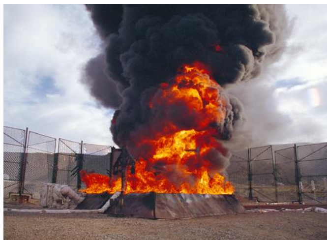
Figure 10: Example of a pool fire [51]
