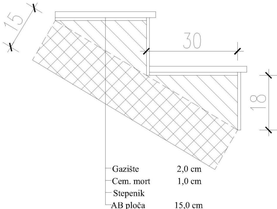
$$\begin{aligned} \operatorname{tg} \alpha &= v_{st} / s_{st} = 18/30 = 0,60 ; \alpha = 30,96^{\circ} \\ h' &= h / \cos \alpha = 15 / \cos 30,96^{\circ} = 17,49 \text{ cm} \end{aligned}$$
