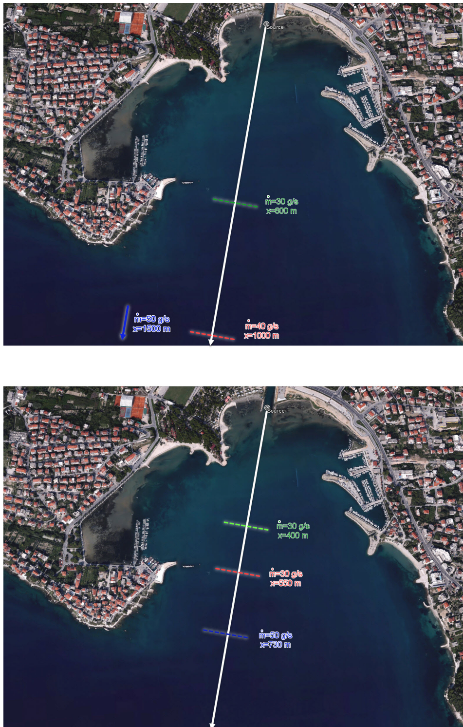
FIGURE 5.47: The seaward extension of the dilution process for c^* = 1 \text{ mg/l} as a function of different estimated river loadings for constant mean velocity (up) and for a decreasing mean velocity with the attenuation factor of \nu = 0.002 \text{ m}^{-1} (down).
