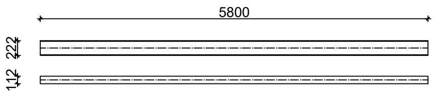
BOČNI SEKUNDARNI NOSAČI IPE 220  $\square$  l=5800mm, kom=88
