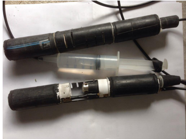
FIGURE A.21: Borehole packers.
