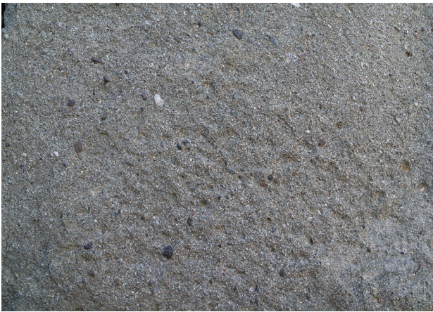
Fig. 7. Volcaniclastic sandstone, macroscopic appearance (photo: B. Djurić)
