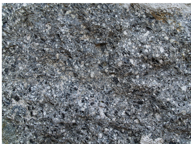
Fig. 4. Hornblende andesite, macroscopic appearance (photo: B. Djurić)
