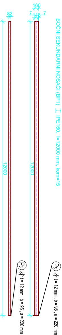
BOČNI SEKUNDARNI NOSAČI (BP2) I IPE160, l=5000 mm, kom=3
