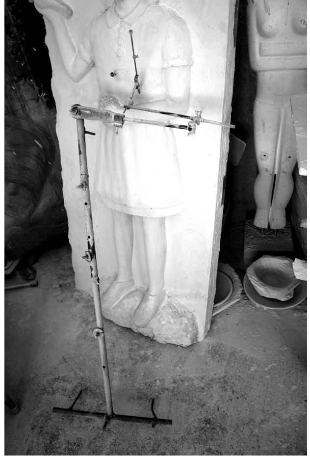
Fig. 27. Pointing machine in the workshop of a portraitist, Tinos, Greece (photo: S. Moureaud)
