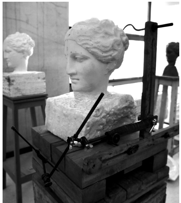
Fig. 28. Pointing machine in the Museum of Marble Craft, Tinos, Greece (photo: S. Moureaud)
