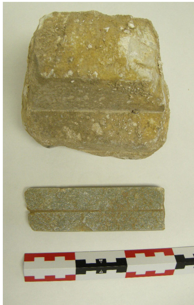
Fig. 12. Two marble blocks showing the cutting line for the production of slabs (photo: Đ. Gobić-Bravar)
