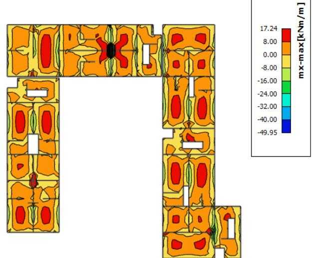
**Slika 11.35.  $M_x$**  **$M_y$  (kritični presjek)**
