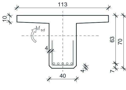
$$\text{C } 40/50 \rightarrow f_{ck} = 40 \text{ MPa} \rightarrow f_{cd} = \frac{f_{ck}}{\gamma_c} = \frac{40}{1.5} = 26,67 \text{ MPa}$$
