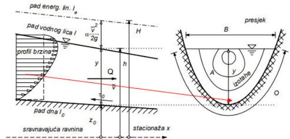
**Jednoliko strujanje:**  $I = I_0 = I_e \quad \bar{v} = \frac{\sqrt{2g}}{\sqrt{c_f}} \sqrt{RI_0}$
