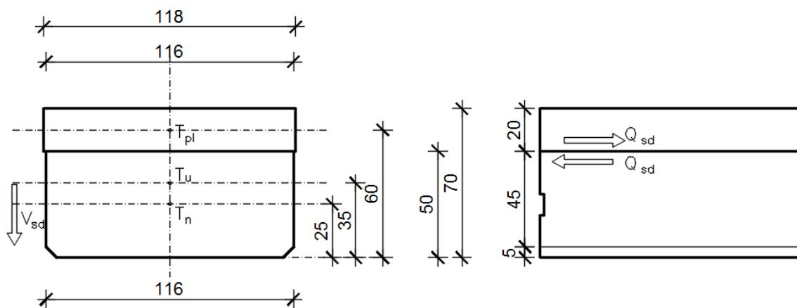
$$\left. \begin{array}{l} A_n = 0.578 \text{ m}^2 \quad h_{t,n} = 0.25 \text{ m} \\ A_{pl} = 0.236 \text{ m}^2 \quad h_{t,pl} = 0.60 \text{ m} \end{array} \right\} \quad A_u = 0.814 \text{ m}^2 \quad h_{t,u} = 0.35 \text{ m}$$
