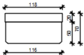
$$\begin{aligned} A &= 0.814 \text{ m}^2 \\ I_y &= 0.0916 \text{ m}^4 \\ I_z &= 0.0331 \text{ m}^4 \\ E &= 34000 \text{ MPa} \end{aligned}$$
