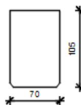
$$\begin{aligned} A &= 0.558 \text{ m}^2 \\ I_y &= 0.0226 \text{ m}^4 \\ I_z &= 0.0295 \text{ m}^4 \\ E &= 34000 \text{ MPa} \end{aligned}$$
