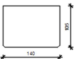
$$\begin{aligned} A &= 1.47 \text{ m}^2 \\ I_y &= 0.135 \text{ m}^4 \\ I_z &= 0.240 \text{ m}^4 \\ E &= 34000 \text{ MPa} \end{aligned}$$
