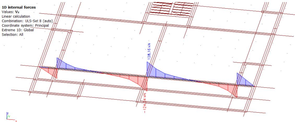
Slika 112 Dijagram poprečnih sila V<sub>z</sub> na gredama**Poprečni presjek grede:**
