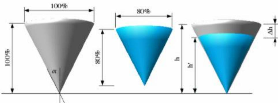
Under the prerequisite of an isotropic shrinkage (expansion) the radius  $r$  and the height  $h$  of a cone shrink (expand) the same percentage:  $h' = k \cdot h$  and  $r' = k \cdot r$  ( $k$  for example 80%)
