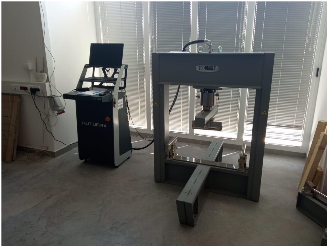
Slika 56: Uređaj AUTOMAX MULTITEST Computerized Control Console
