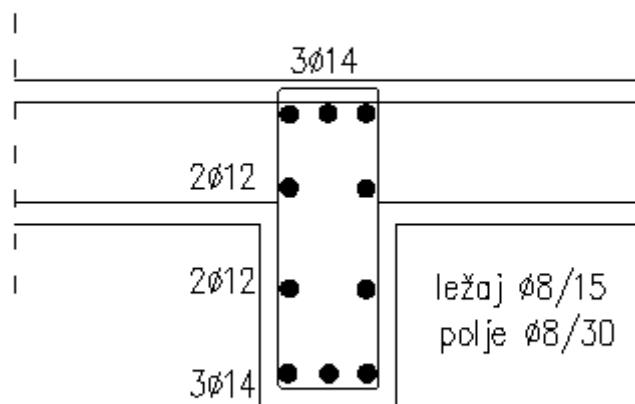
Slika 6.30. Detalj armiranja grede G502, G402, G302, G505, G405, G305 b/h=20/45
