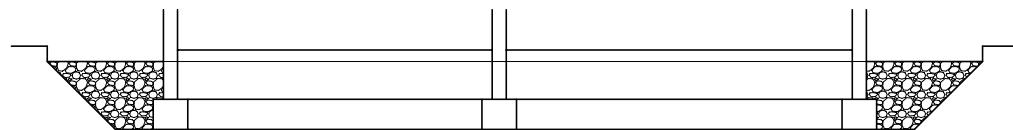
$$V_{\text{uk,vz}} = V_{\text{ši}} - V_{\text{tt}} - V_{\text{nz}} - V_{z2} - V_{z1} = 190 - 11.97 - 6.28 - 33.39 - 66.64 = 71.72 \text{ m}^3$$
