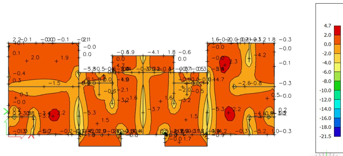
Slika 30. Armatura u ploči smjer  $As,x-x$  ( $\text{cm}^2/\text{m}$ ) za GSN1
