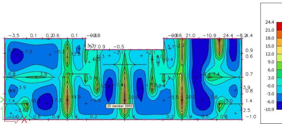
Slika 56. Armatura u ploči smjer As,x-x ( $\text{cm}^2/\text{m}$ ) za GSN1
