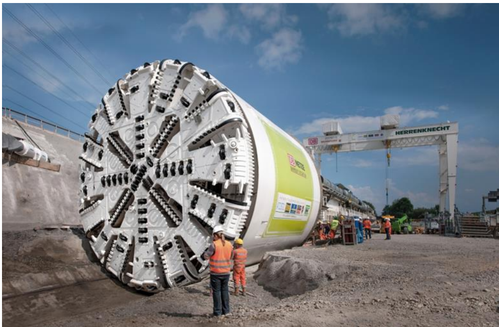
Slika 2.1: Herrenknecht Multi-Mode Tunnel Boring Machine [2]
