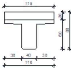
$$\begin{aligned} A &= 0.557 \text{ m}^2 \\ I_y &= 0.0438 \text{ m}^4 \\ I_z &= 0.0268 \text{ m}^4 \\ E &= 34000 \text{ MPa} \end{aligned}$$
