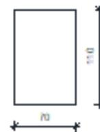
$$\begin{aligned} A &= 1.000 \text{ m}^2 \\ I_y &= 10.0 \text{ m}^4 \\ I_z &= 0.1302 \text{ m}^4 \\ E &= 34000 \text{ MPa} \end{aligned}$$
