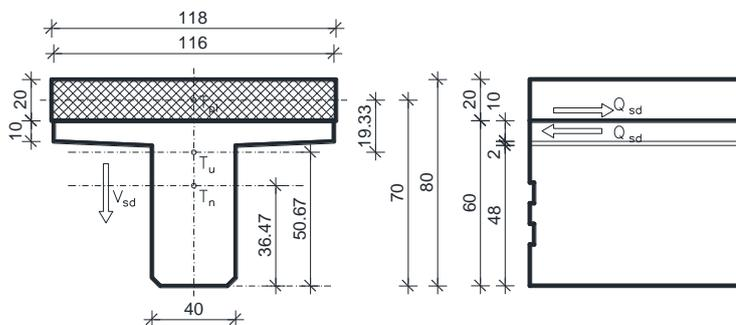
$$\left. \begin{array}{l} A_n = 0.321 \text{ m}^2 \quad h_{t,n} = 0.365 \text{ m} \\ A_{pl} = 0.236 \text{ m}^2 \quad h_{t,pl} = 0.70 \text{ m} \end{array} \right\} A_u = 0.558 \text{ m}^2 \quad h_{t,u} = 0.507 \text{ m}$$
