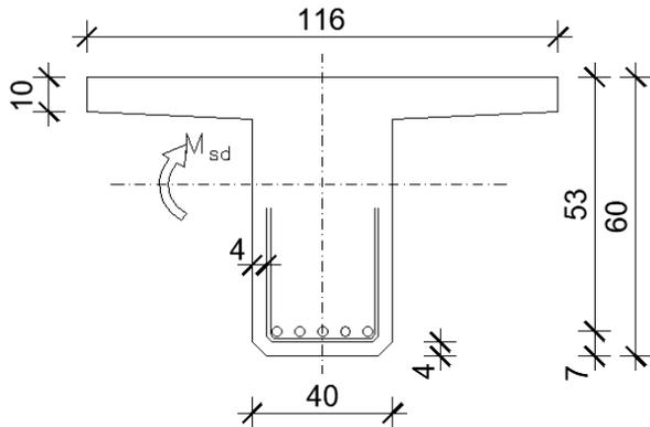
$$V_{g1} = 65,68 \text{ kNm}; \quad V_{g2} = 48,16 \text{ kNm}$$
