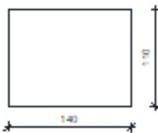
$$\begin{aligned} A &= 1.820 \text{ m}^2 \\ I_y &= 10.0 \text{ m}^4 \\ I_z &= 0.2563 \text{ m}^4 \\ E &= 34000 \text{ MPa} \end{aligned}$$
