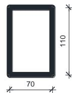
$$\begin{aligned}A &= 0.77 \text{ m}^2 \\I_y &= 10.0 \text{ m}^4 \\I_z &= 0.1302 \text{ m}^4\end{aligned}$$
