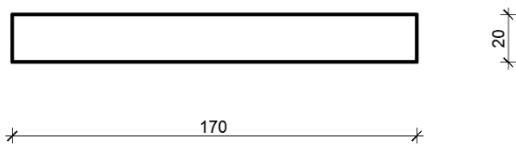
$$\begin{aligned}A &= 0.34 \text{ cm}^2 \\I_y &= 0.0011 \text{ m}^4 \\I_z &= 0.0819 \text{ m}^4 \\E &= 34000 \text{ MPa}\end{aligned}$$
