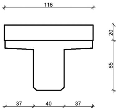
$$\begin{aligned}A &= 0.5718 \text{ cm}^2 \\I_y &= 0.0321 \text{ m}^4 \\I_z &= 0.0421 \text{ m}^4 \\E &= 34000 \text{ MPa}\end{aligned}$$
