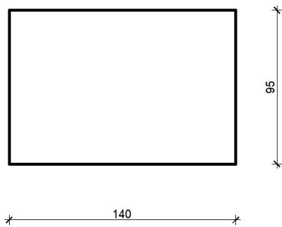
$$\begin{aligned}A &= 1.33 \text{ cm}^2 \\I_y &= 0.1000 \text{ m}^4 \\I_z &= 0.2172 \text{ m}^4 \\E &= 34000 \text{ MPa}\end{aligned}$$
