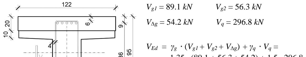
$$V_{Ed} = \gamma_g \cdot (V_{g1} + V_{g2} + V_{\Delta g}) + \gamma_q \cdot V_q = \\ = 1.35 \cdot (89.1 + 56.3 + 54.2) + 1.5 \cdot 296.8$$
