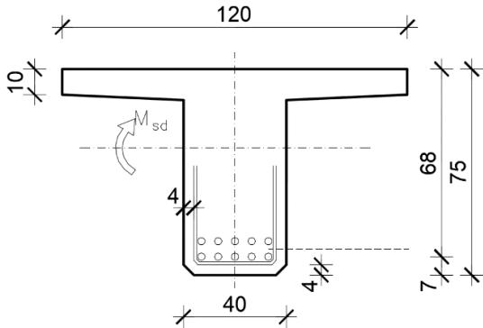
$$C \quad 30/37 \Rightarrow f_{ck} = 30.0 \text{ MPa} \Rightarrow \\ f_{cd} = \frac{f_{ck}}{\gamma_c} = \frac{30.0}{1.5} = 20.0 \text{ MPa} \\ B450C \Rightarrow f_{yk} = 450.0 \text{ MPa} \Rightarrow \\ f_{yd} = \frac{f_{yk}}{\gamma_s} = \frac{450.0}{1.15} = 391.3 \text{ MPa}$$
