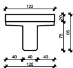
$$\begin{aligned}A &= 0.630 \text{ m}^2 \\I_y &= 0.023 \text{ m}^4 \\I_z &= 0.046 \text{ m}^4 \\E &= 34000 \text{ MPa}\end{aligned}$$
