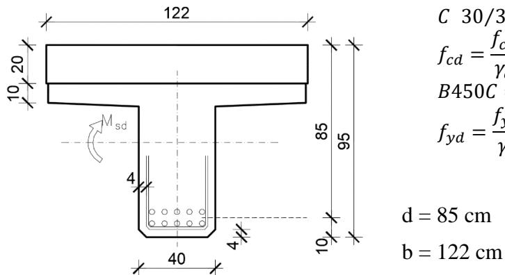
$$C \ 30/37 \Rightarrow f_{ck} = 30.0 \text{ MPa} \Rightarrow \\ f_{cd} = \frac{f_{ck}}{\gamma_c} = \frac{30.0}{1.5} = 20.0 \text{ MPa} \\ B450C \Rightarrow f_{yk} = 450.0 \text{ MPa} \Rightarrow \\ f_{yd} = \frac{f_{yk}}{\gamma_s} = \frac{450.0}{1.15} = 391.3 \text{ MPa}$$
