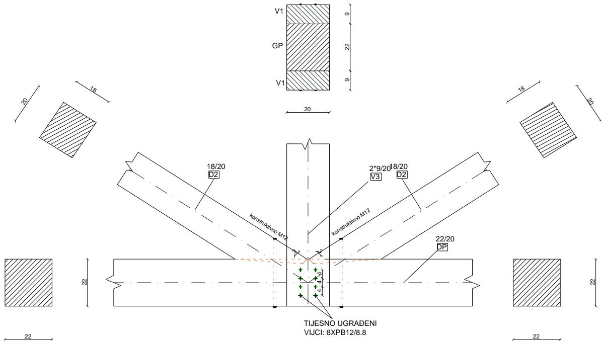
$$f_{c,a,d} = \frac{f_{c,0,d}}{\sqrt{\left(\frac{f_{c,0,d}}{2 \cdot f_{c,90,d}} \cdot \sin^2 \alpha\right)^2 + \left(\frac{f_{c,0,d}}{2 \cdot f_{v,d}} \cdot \sin \alpha \cdot \cos \alpha\right)^2 + \cos^4 \alpha}}$$
