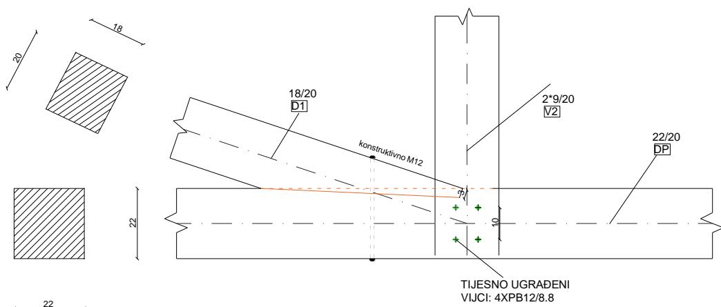
$$f_{c,a,d} = \frac{f_{c,0,d}}{\sqrt{\left(\frac{f_{c,0,d}}{2 \cdot f_{c,90,d}} \cdot \sin^2 \alpha\right)^2 + \left(\frac{f_{c,0,d}}{2 \cdot f_{v,d}} \cdot \sin \alpha \cdot \cos \alpha\right)^2 + \cos^4 \alpha}}$$
