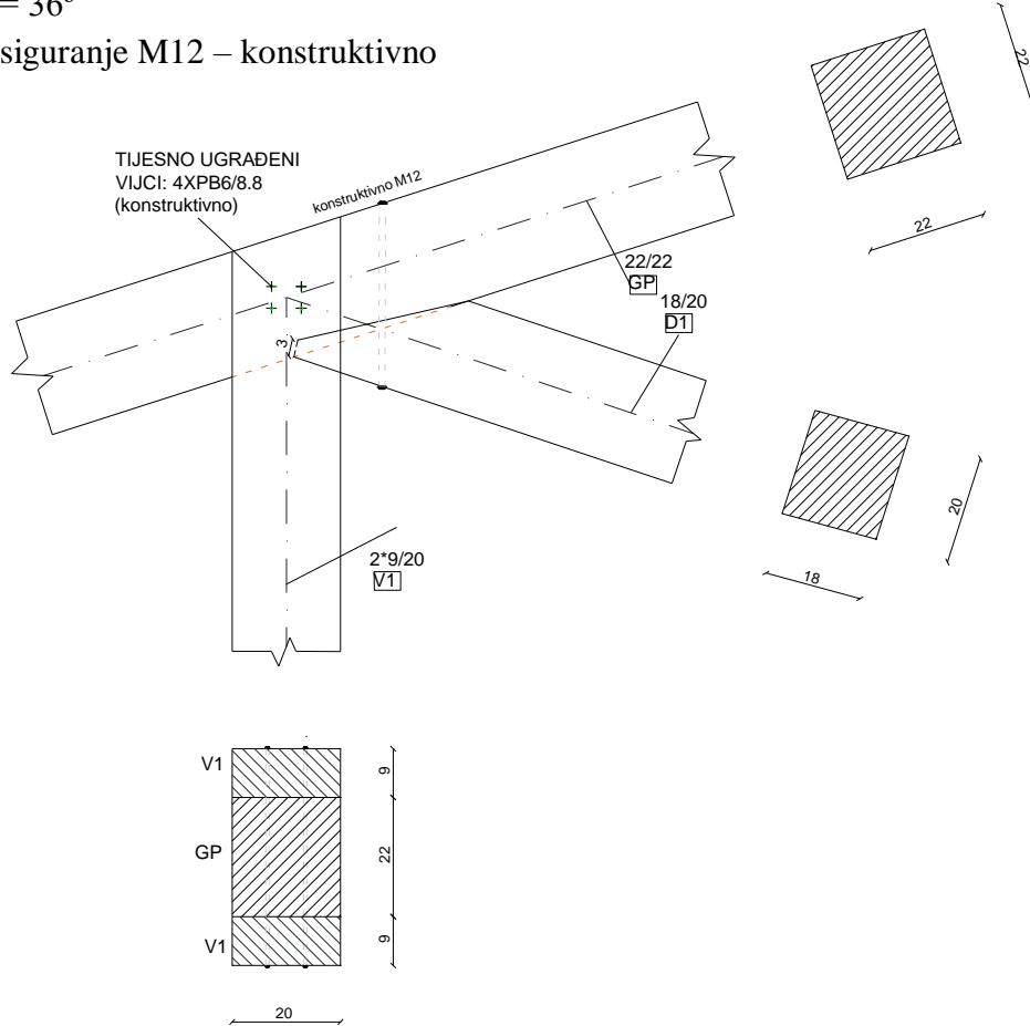
$$f_{c,a,d} = \frac{f_{c,0,d}}{\sqrt{\left(\frac{f_{c,0,d}}{2 \cdot f_{c,90,d}} \cdot \sin^2 \alpha\right)^2 + \left(\frac{f_{c,0,d}}{2 \cdot f_{v,d}} \cdot \sin \alpha \cdot \cos \alpha\right)^2 + \cos^4 \alpha}}$$
